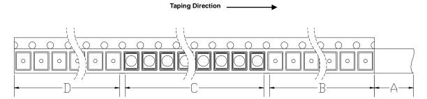
A: Top Cover Tape, 300mm; B: Leader, Empty, 200mm; C: 1000 Lamps Loaded; D: Trailer, Empty, 200mm.
